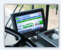
Vehicle operators can also selfregulate their headway spacing by providing information on their Transit Control Head (TCH).
